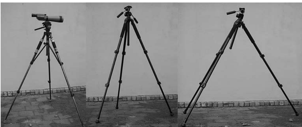
The left hand tripod has the legs attached to the centre column, the legs can only be pulled out a certain distance, and they always come out evenly. The right hand tripod has independent legs, they come out separately, and each leg can come out further than the first place that they stop, the last photo shows one leg pulled out further than usual.
